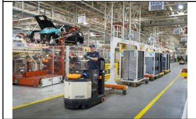
Fuel cell powered materials handling equipment at BMW Manufacturing Plant – Greer, South Carolina
