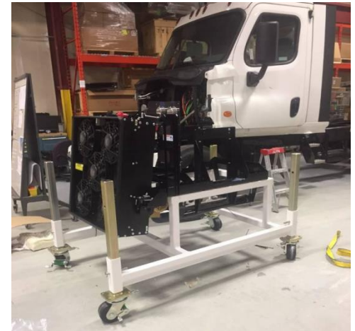
Fuel Cell support cradle assembly with thermal management system and test rig in front of DTNA glider chassis.
